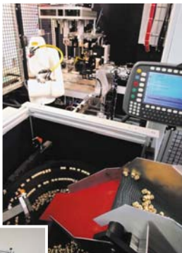
Distribution of pieces by vibrating bowl, orientation and deposition by 6-axis robot
