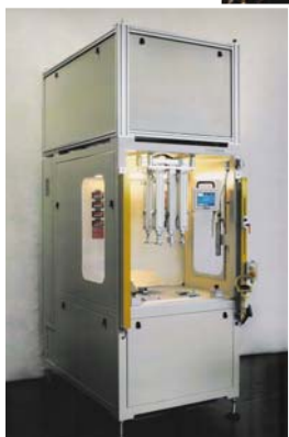
Manual-loading machine with operator protection by non-physical barriers
