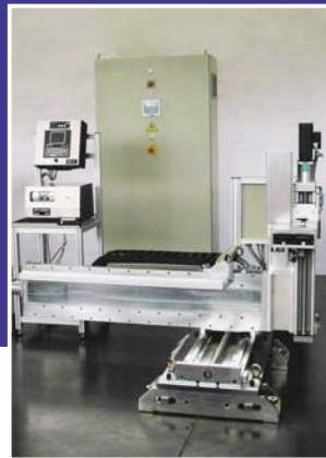
Fully stainless steel robot for sterile room
