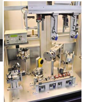
Tooling for checking fluidtightness with camera code reading
